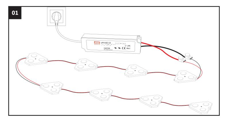
Before installation, check the entire chain of LED modules for light intensity and color consistency.
